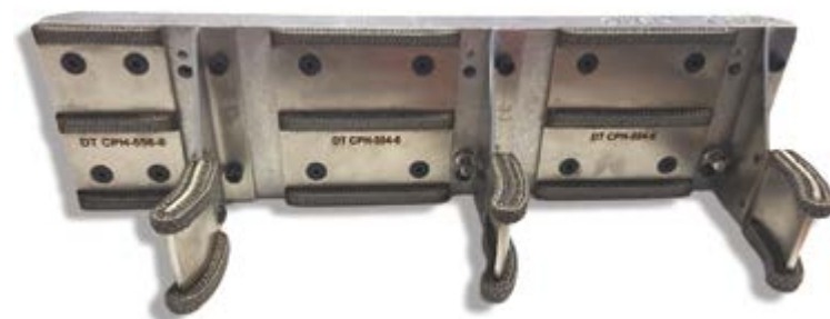
Triple gob Vortex Sweepout Assembly with stainless steel braid.
